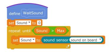
If Sound is larger than Max, repeatedly put the values of the sound sensor in Sound; if Sound is not larger than Max, the program will stop repeated actions, and execute the successive command instead.
