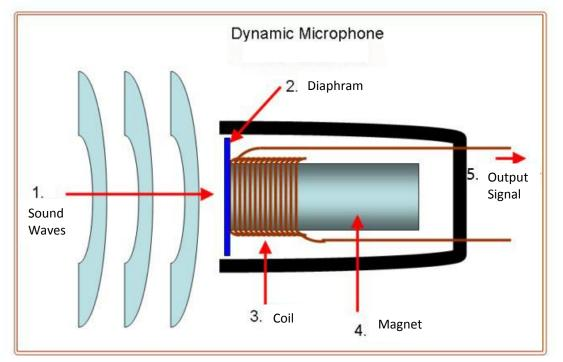
When sound waves propel the coil connected on the vibration diaphragm, make it move back and forth in the magnetic field generated by the magnet, bringing the change of current in the coil (Faraday's Law, Lenz's Law).
