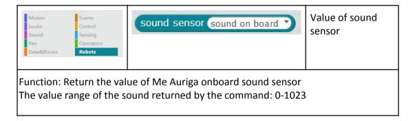
What the command sends back is the volume of sound sensor. By convention, we should create a variable called Sound first.
