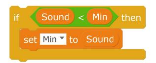
Never forget to handle the initial value of the maximal and minimal values at the very beginning of the program. In doing so, the minimal value will not be 0 for long.
