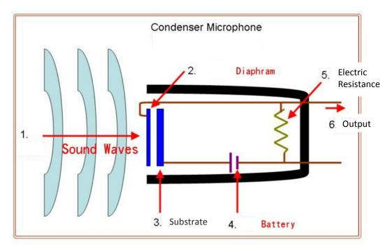
Capacity stored in the condenser varies because of different distances between two polar plates. When sound waves change the distance of condenser plates, the capacity will be absorbed or the capacity stored in the condenser will be discharged by the battery. In doing so, the change of sound will be reflected in the output voltage.
