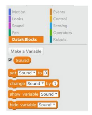
Then repeatedly put the values of sensor into Sound, and the command we use is "Set Sound to Sound Sensor onboard".
