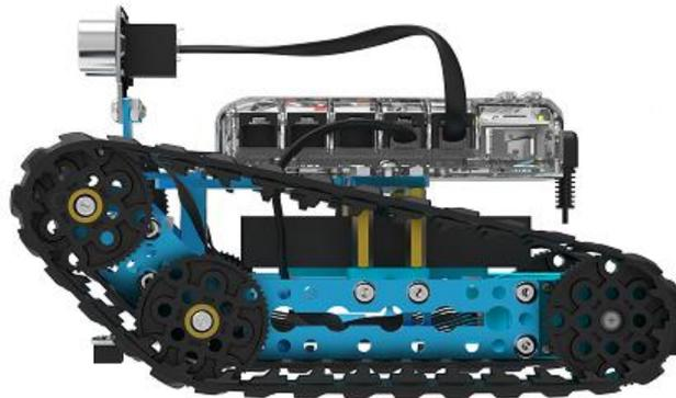
The position of the line-follower sensor being assembled will affect the ability of the robot to follow the track. Different track shapes will then require different installation positions in order for it to be most efficient.
