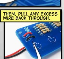
THE LOOPS SERVE AS A STRAIN RELIEF FOR THE WIRES.
