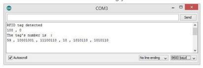
When the RFID reader senses a card, it starts by printing "RFID tag detected" on the Serial Monitor. The next line verifies the card type. In normal use, this would be unnecessary. The next two lines print out the data stored in the card, in this case an ID identifying the specific tag scanned.
