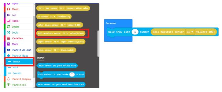
**Result:** The value of the current soil moisture display on the OLED module.
