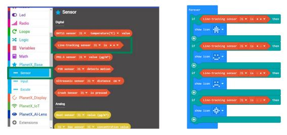
**Result:** Different icons display on the Micro:bit in accordance with the different status detected by the tracking module.
