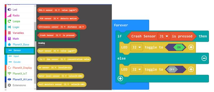
Result: The LED lights on if the crash switch was pressed or it lights off.
