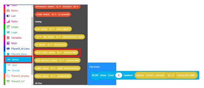
**Result:** The current value of the water level displays on the OLED screen.
