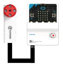
**Result:** When button A is pressed, the motor connected to port M1 starts to move with 50% of speed. When button B is pressed, the motor stops. When Micro:bit logo is pressed, The motor will start to move in it's first position automatically.
