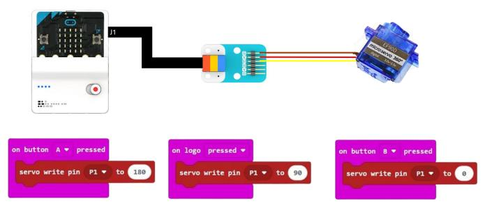
Result: The Servo Motor change it's direction on buttons press and stops by touching Micro:bit logo.
