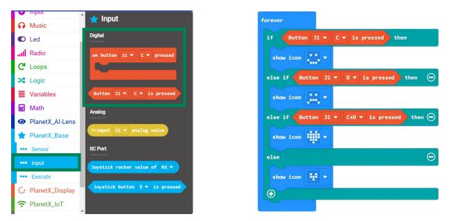
**Result:** The icons display on the Micro:bit accordingly with the order given by pressing button A or B or A+B.
