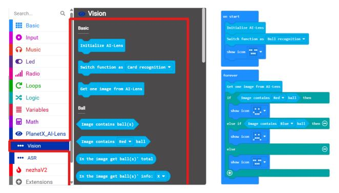
**Result:** A smile face displays on the Micro:bit if the the blue ball is recognized by the AI lens and a sad face display on the Micro:bit if it recognizes a red ball. A poker face will be displayed when none of the balls detected.
