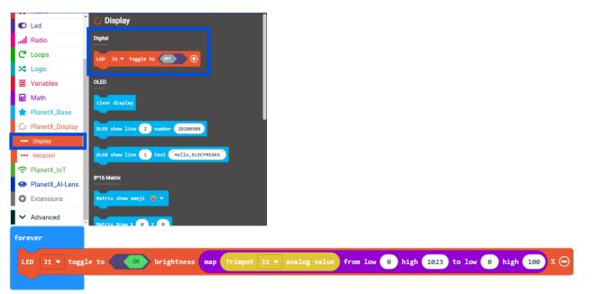
**Result:** The brightness is adjusted by the potentiometer by using a map block which can match Analog Data from 0 to 1023 with brightness from 0 to 100%.
