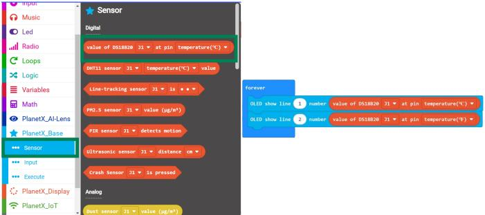
**Result:** The value detected by 18B20 temperature sensor displays on the OLED screen in Fahrenheit and Celsius.
