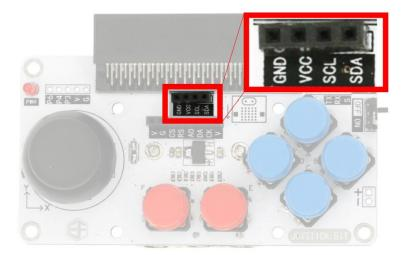
4) SPI Communication Connector: V / G / CS / RS / AO / DA / CK correspond to the connector of TFT 1.8 inch LCD module. It can directly compatible with TFT 1.8 inch LCD module, including SPI communication connector on micro:bit board.
